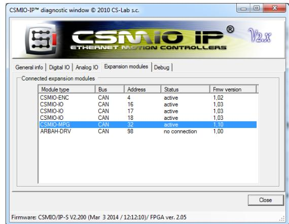
If connections are correct, the CSMIO-MPG module should appear on the list of modules detected by our controller.
