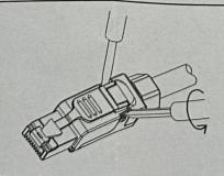
Step 2: Insert the slotted screwdriver into the slot and rotate to open the jaws.
